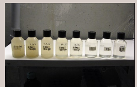
Samples of road runoff before, during and after treatment in a 50 m long Dual Porosity Filter located belowground in a park in Ørestad. Bottle 1 (most left) contains inlet water, while bottle 8 is the treated outlet water. The 6 bottles in between are sampled after passage of 1 m, 10 m, 20 m, 30 m, 40 m and 49 m of the filter. Photo: Marina Bergen Jensen.
